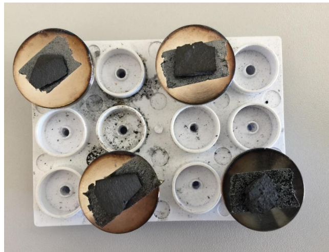
Figure 4.5 Cement chips for SEM tests
