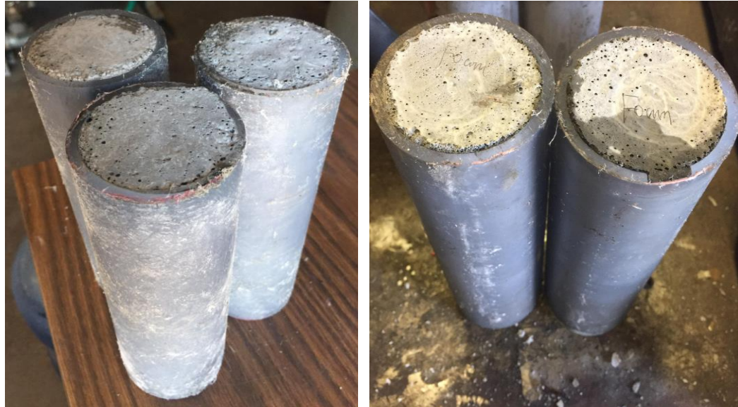
Figure 5.25 Hardened foam cement with the densities of 12 ppg (left) and 14 ppg (right)
