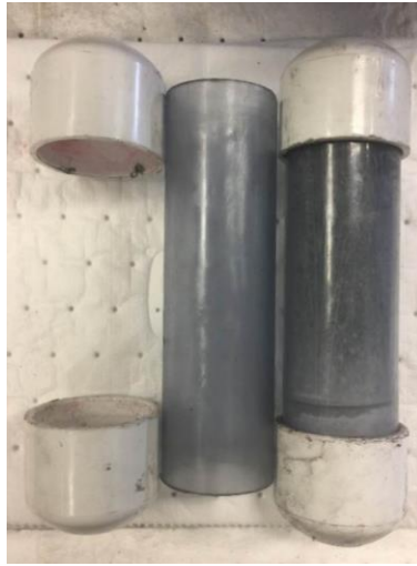
Figure 3.2 PVC molds for curing cement
