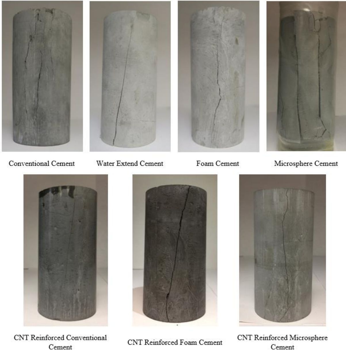
Figure 5.7 Cement specimens at failure
