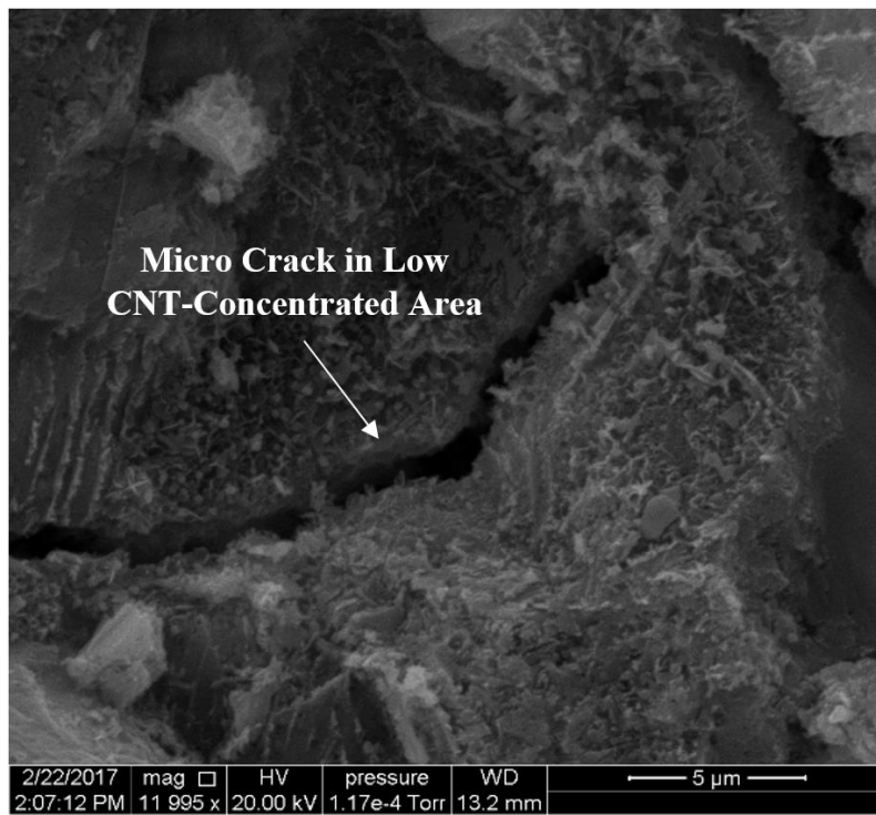
Figure 5.21 SEM image of a micro crack in low CNT concentrated area
